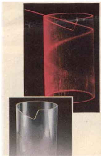
Fig. 3. Internal reflection tube (Photo courtesy of CENCO)
