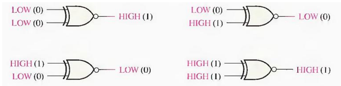
Fig.(2-20) All possible logic levels for an exclusive-NOR gate.
