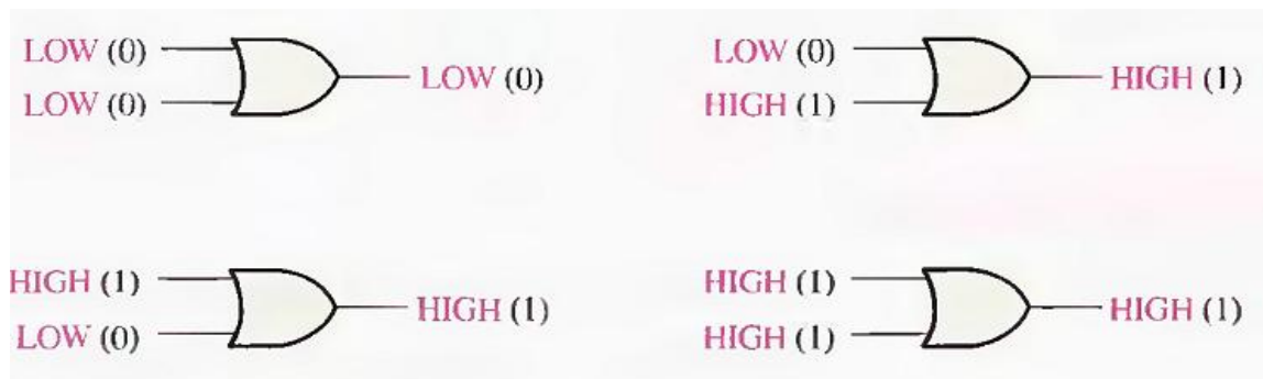
Fig.(2-8) All possible logic levels for a 2-input OR gate.
